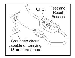
therapy spa. First, turn on the spa by pressing the jet button on the console (see USING THE CONTROLS on page 12). Once the spa is running, press the GFCI "test" button. The spa should shut off. Press the "reset" button. The spa should resume normal operation. If the spa continues to run after the "test" button is pressed, the GFCI is damaged. Do not use the spa until the GFCI has been repaired or replaced by a qualified electrician.
